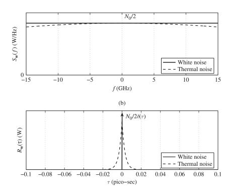
Figure 23: (a) The PSD  $(S_N(f))$ , and (b) the autocorrelation  $(R_N(\tau))$  of noise. (Assume G = 1/10 (mhos), T = 298.15 K, and  $t_0 = 3 \times 10^{-12}$  seconds.) [11, Fig. 3.11]
