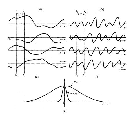
Figure 22: Autocorrelation functions for a slowly varying and a rapidly varying random process [9, Fig. 11.4]
